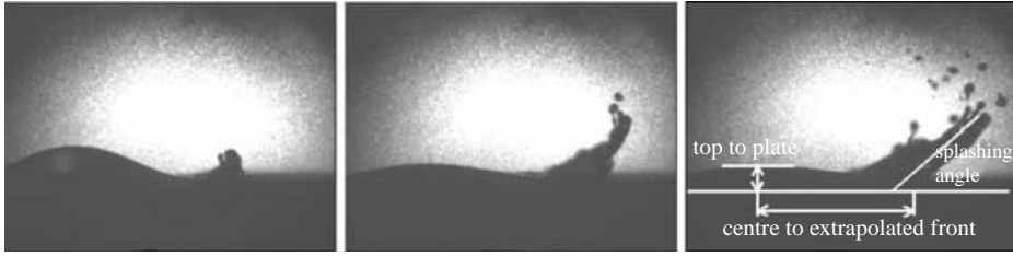
FIGURE 1. Impact on the 0.035 mm obstacle (from left to right 1000, 1500 and 1750 \mu\text{s} after impact). A sketch of the measurement of the angle of deviation is shown on the right-hand figure.
