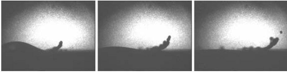
FIGURE 2. Impact on the 0.07 mm obstacle (from left to right: 1000, 1500, 2000 \mu\text{s} after impact).
