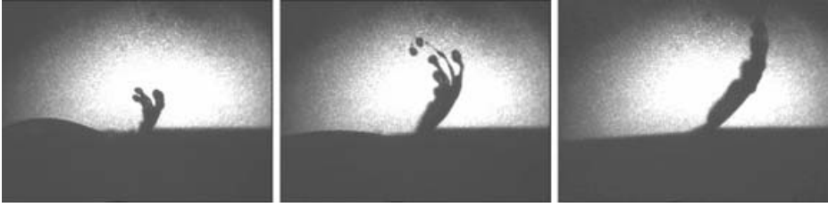
FIGURE 3. Impact on the 0.2 mm obstacle (from left to right: 1000, 1500, 2500 \mu s after impact).
